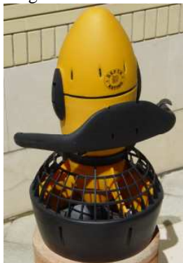
Fig. 3. Sea-scooter which used as the ROV actuators
