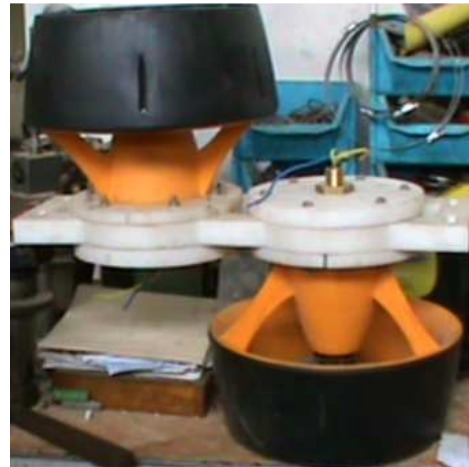
Fig. 4.b. Sea-scooters are waterproofed and assembled to the thruster chassis
