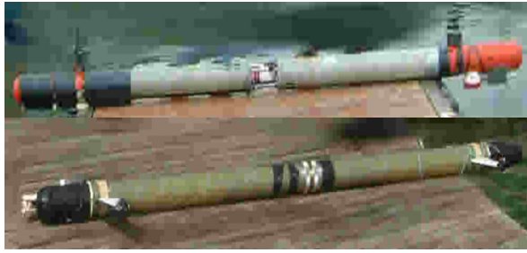
Fig. 1. The first (top) and second (bottom) version of the Fòlaga. The main difference between the two versions is in the vertical propulsion pumps: in the first version there is one pump placed at the center of the vehicle, in the second version there are two pumps placed at the bow and stern of the vehicle respectively.
