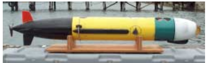
Fig. 5. REMUS Vehicle with Sidescan Sonar and ADCP Transducers
