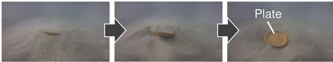
Fig. 8 Sediment removal test for a plate
