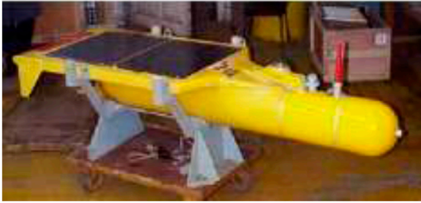
FIGURE 1 | Engineering prototype of the SAUV.
