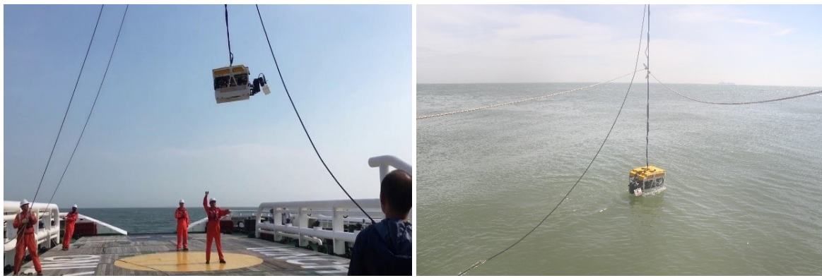
Figure 22. Search and rescue ROV is dropped into water.
