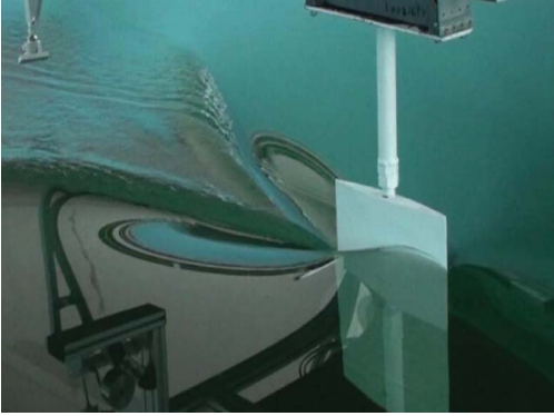
Figure 7c. Hydrodynamic support, immersion I = 0.55 m and speed v = 1.5 m/s.
