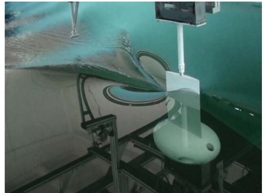
Figure 11b. ROV-hydrodynamic support system, immersion I = 0.55 m and speed v = 1.5 m/s.
