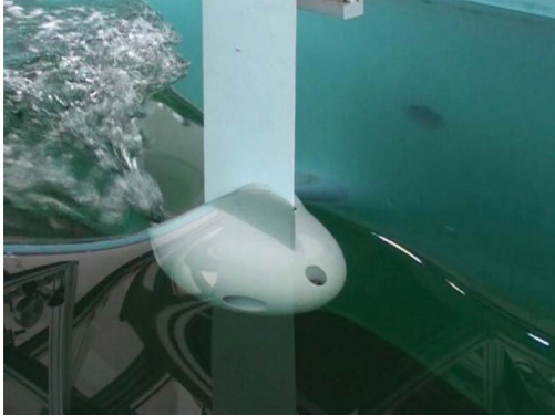
Figure 10b. ROV-hydrodynamic support system, immersion I = 0.05 m and speed v = 1.75 m/s.
