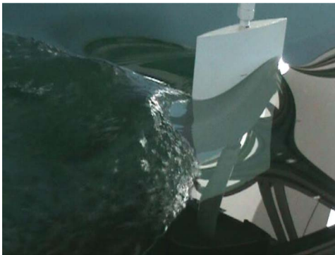
Figure 6a. Hydrodynamic support, immersion I = 0.55 m and speed v = 1 m/s.
