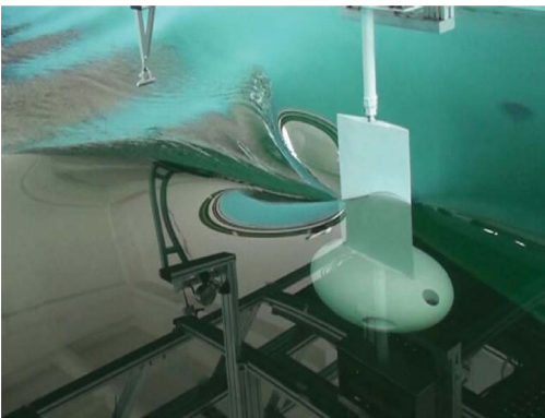
Figure 12b. ROV-hydrodynamic support system, immersion I = 0.35 m and speed v = 1.5 m/s.
