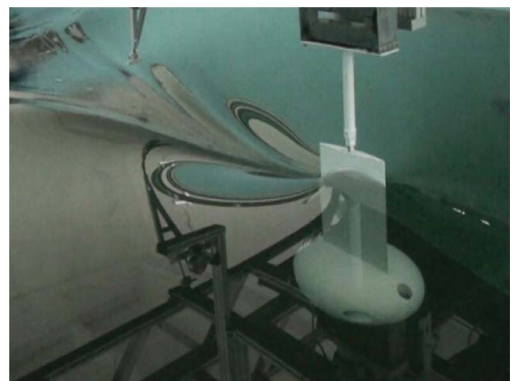
Figure 11c. ROV-hydrodynamic support system, immersion I = 0.55 m and speed v = 2 m/s.
