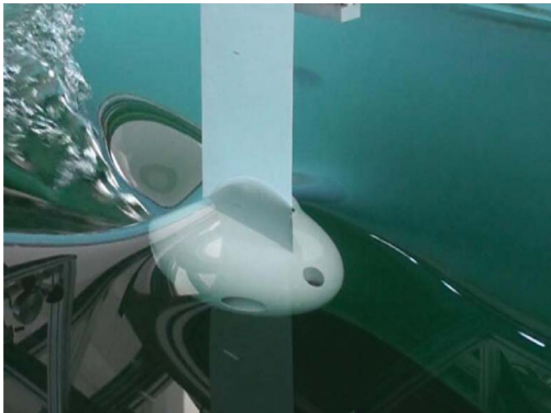
Figure 10c. ROV-hydrodynamic support system, immersion I = 0.05 m and speed v = 2 m/s.
