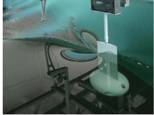
Figure 12c. ROV-hydrodynamic support system, immersion I = 0.55 m and speed v = 1.5 m/s.
