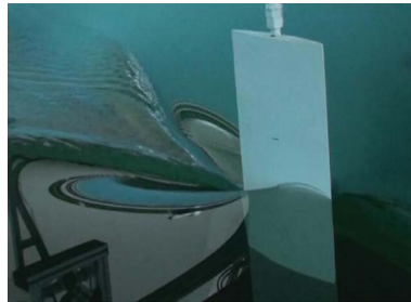
Figure 7b. Hydrodynamic support, immersion I = 0.35 m and speed v = 1.5 m/s.
