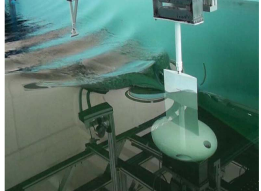
Figure 11a. ROV-hydrodynamic support system, immersion I = 0.55 m and speed v = 1 m/s.
