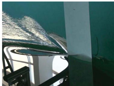
Figure 7a. Hydrodynamic support, immersion I = 0.05 m and speed v = 1.5 m/s.
