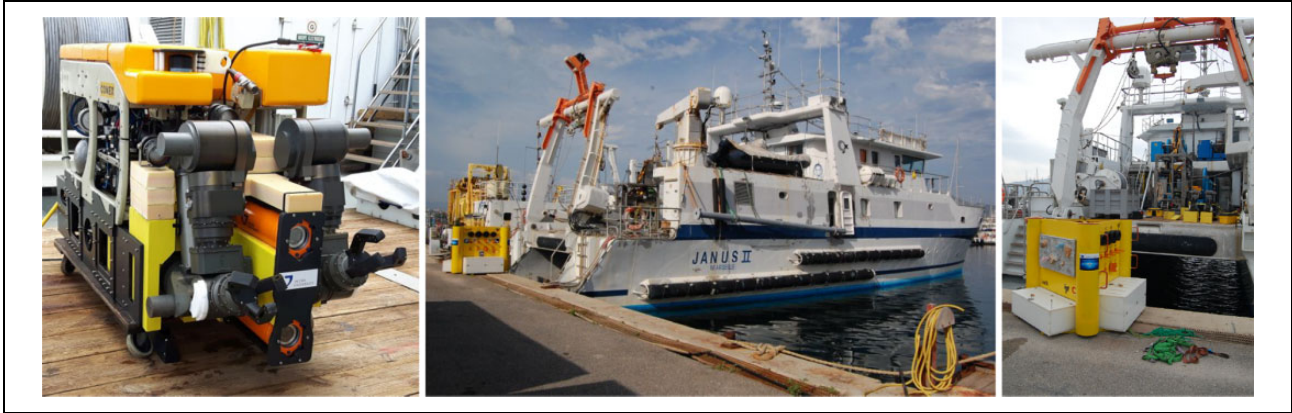
Figure 1. Our navigation system has been employed at a high TRL of 6. It was tested, for example, in two extensive field trials off the shore in Marseille. In addition to the vision system to aid the navigation (left), the setup in these trials consists of an Apache ROV extended a dual arm setup, which is deployed from the COMEX Janus II vessel (center). A mock-up panel structure is used to test different application scenarios (right). TRL: technology readiness level; ROV: remotely operated vehicle.
