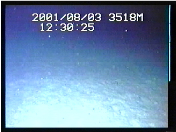
Figure 11. TV Image Transmitted via Acoustic Telemetry from 3,518m
