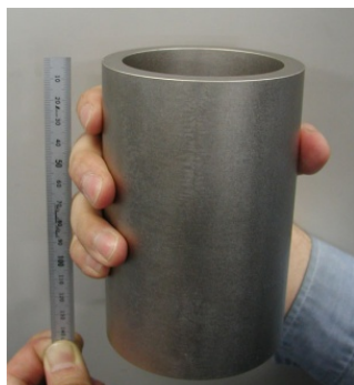
Figure 2. The Prototype Pressure Vessel made by Mg Alloy (Tube Part)
