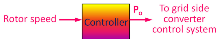
Figure 8. Power Signal Feedback Control Block Diagram.
