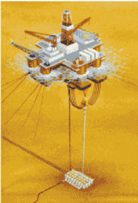
Figure 1: Green Canyon free standing production riser
