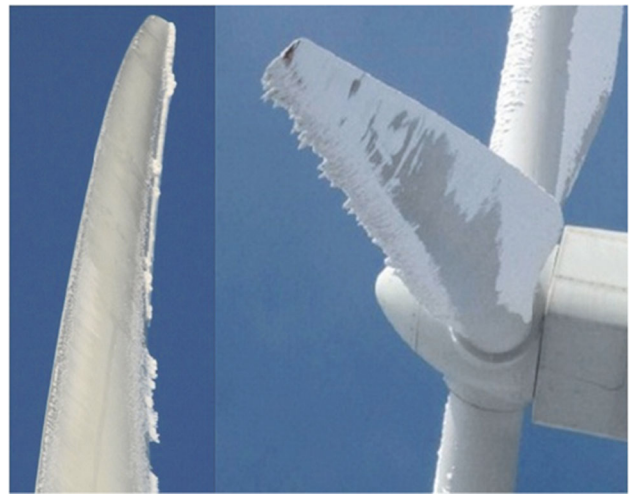
Fig. 11 The ice accumulation on the surface of the wind turbine blade [84]
