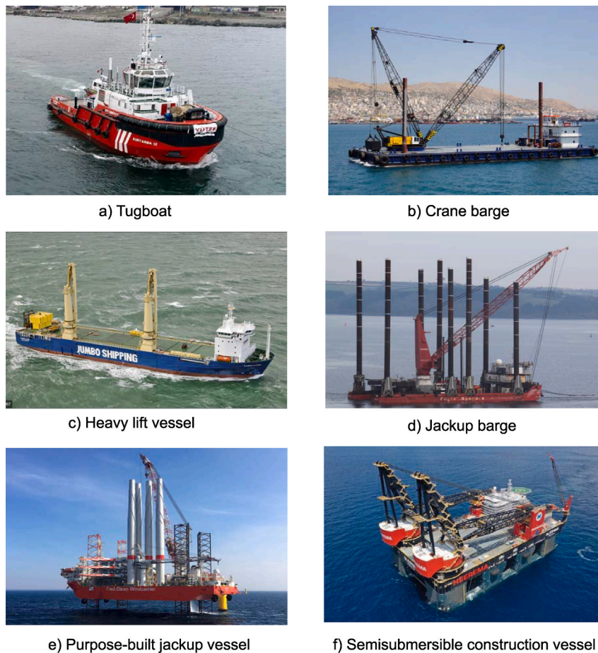
Fig. 5. Common vessels used in OWT installation [153–156] (photo courtesy of Damen Shipyards Group, Spanopoulos Group and Fred Olsen ASA).
