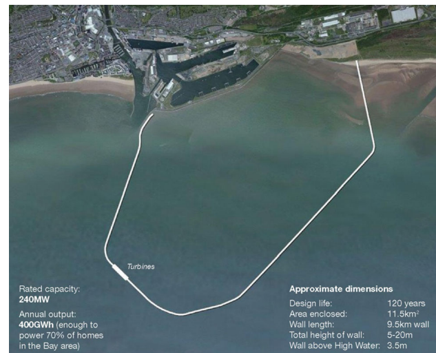
Fig. 10 Map of the proposed Swansea tidal lagoon. Sourced from Tidal Lagoon Swansea Bay plc (2015)
