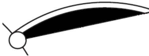
Figure 9.5. Proposed blade alteration
