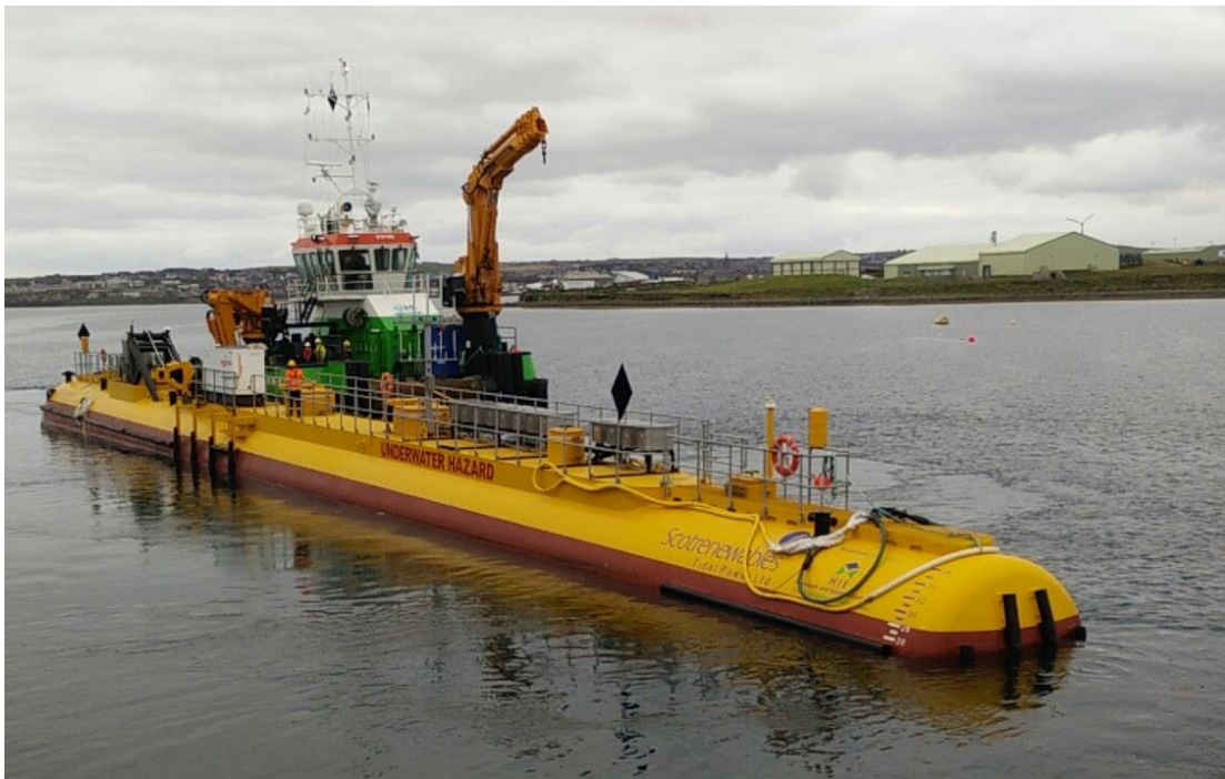
Figure 18: Multi-functional work vessels such as multi-cats are capable of precise movements of platforms in close-quarters and have capacity to tow turbines alongside owing to low well fendered free-board.
