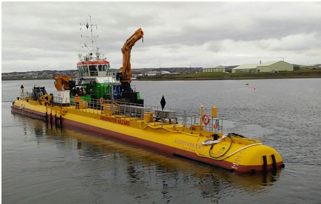
Figure 14: Multi-functional work vessels such as multi-cats are capable of precise movements of platforms in close-quarters and have capacity to tow turbines alongside owing to low well fendered free-board.
