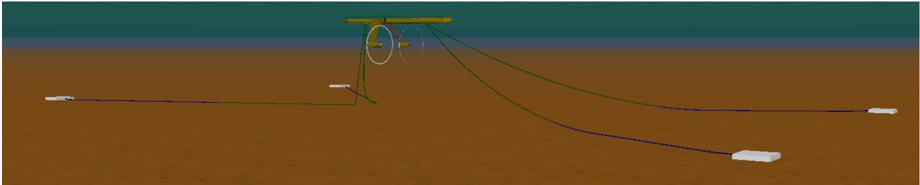
Figure 5 Orbital O2 mooring system operating in tide (green lines are 95mm Studlink chain, blue lines are 115mm studlink)
