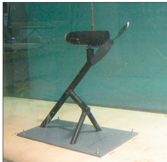
Figure 15. Universal turbine model in situ during an S1 test.
