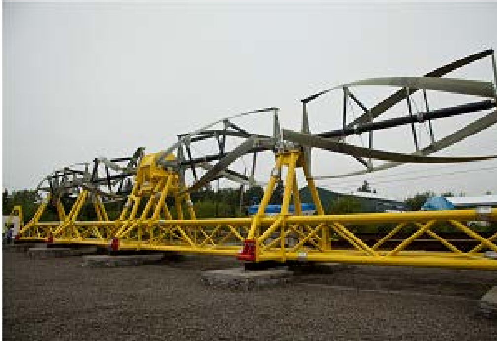
Figure 2. Example tidal generator consisting of series-connected Gorlov turbines
