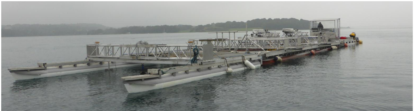
Figure 14: Field testing rig used for still water towing and stationary testing. Source QUB.
