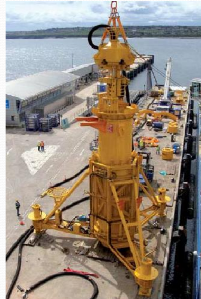
BSD 3000 11 m Monopiles Vouth Tidal Turbines Orkney. Source: Bauer
