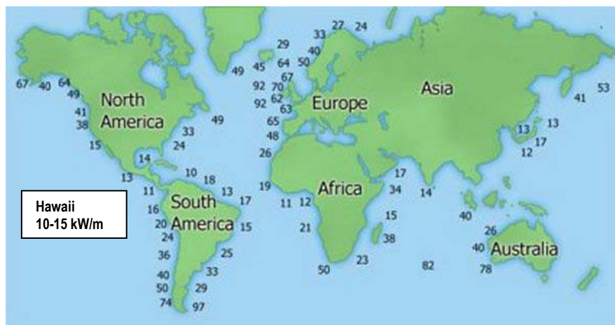
Figure 4: Wave Energy Levels in kW/m Crest Length Courtesy of the European Ocean Energy Association
