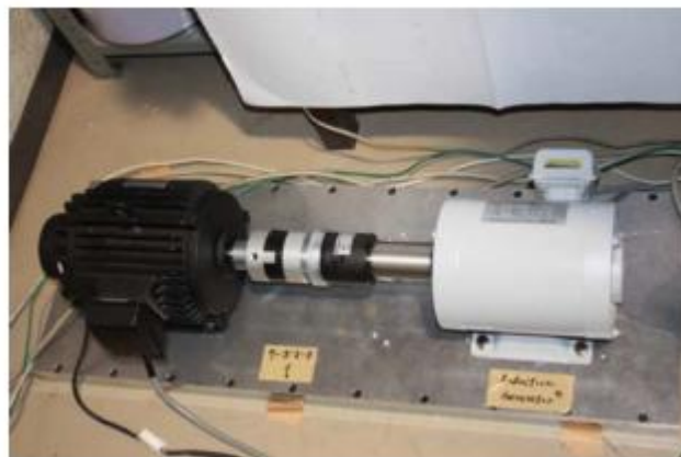
Fig.6: The experimental model of a tidal turbine induction generator/motor.
