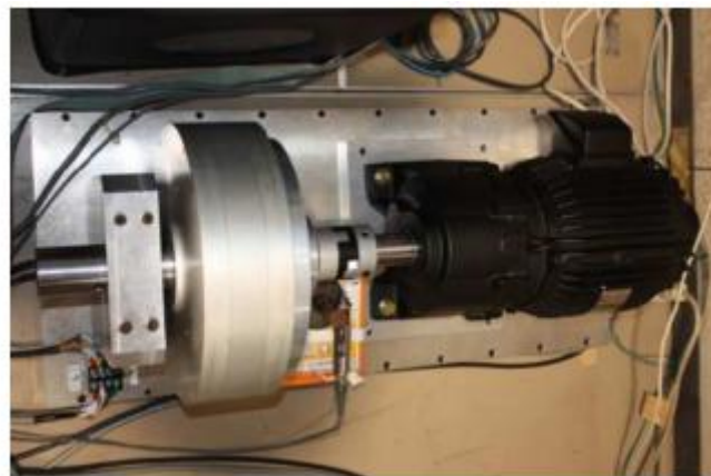
Fig:5: offshore wind generator experimental turbine model
