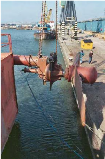
Figure 11: Submergence test for the powertrain on the quayside at Swansea.
