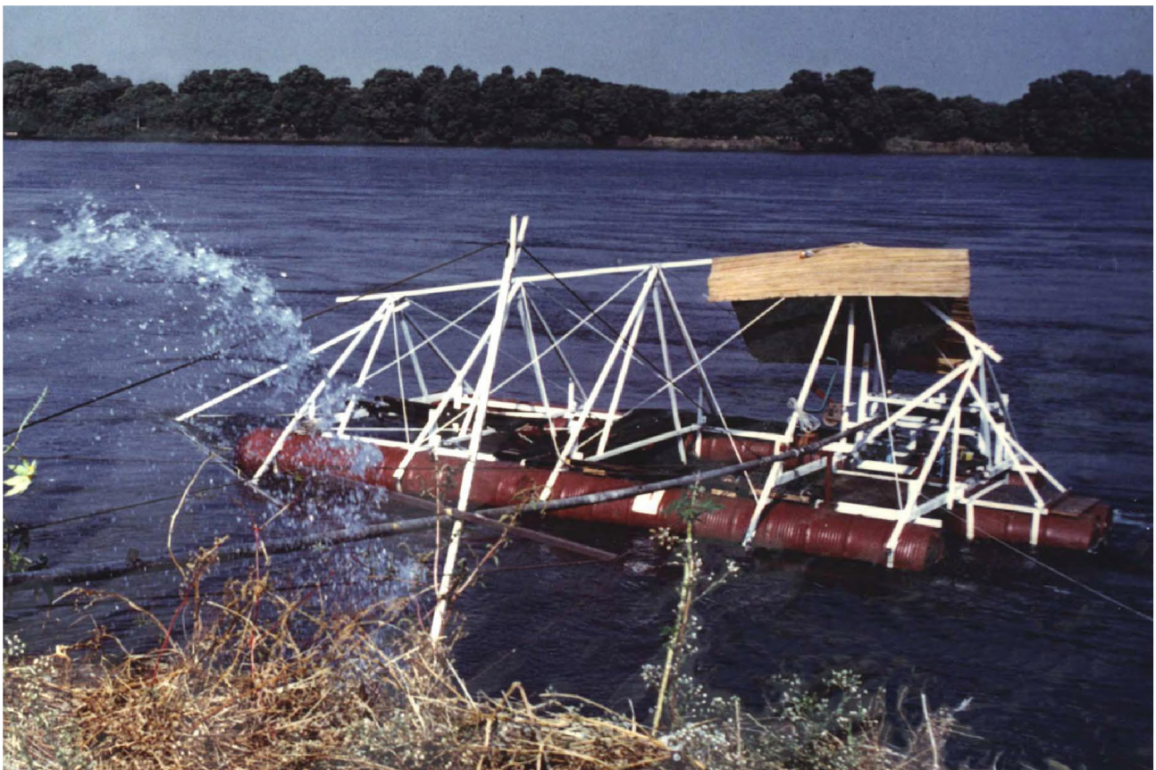
Figure 1: River current turbine on the Nile, Sudan, 1982
