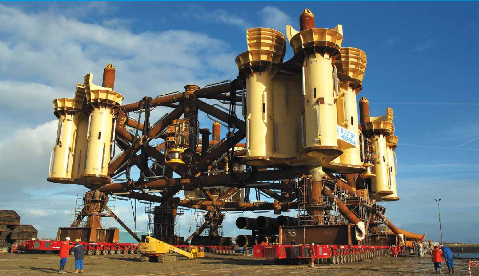
7,000 ton Capacity Template Leveling System
