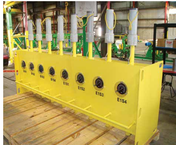
Subsea ROV Grouting and Packer Inflation Panel
