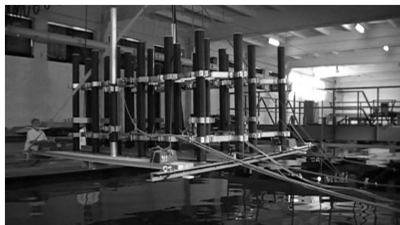
Fig. 9. Testing the submarine breakwater prototype in the towing tank of the Ship Hydromechanics Division, Ship Design and Research Center SA, Gdańsk, Poland [22]
