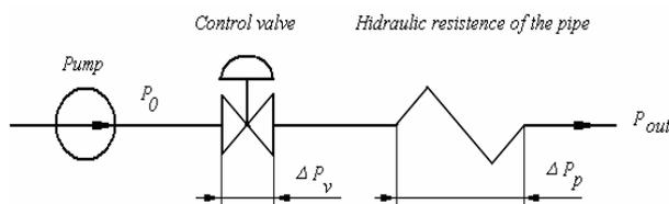
Fig. 5. The structure of the hydraulic system with control valve
