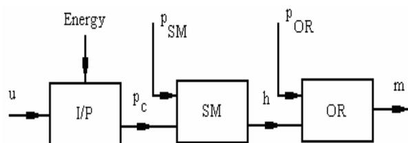
Fig. 1. The structure of the control valve
