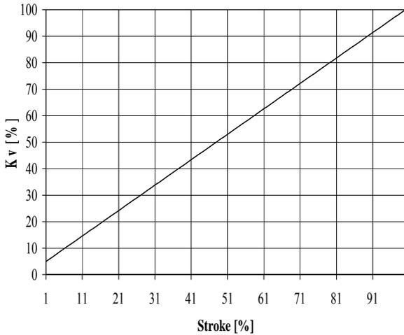
Fig. 6. The intrinsic characteristic of the control valve
