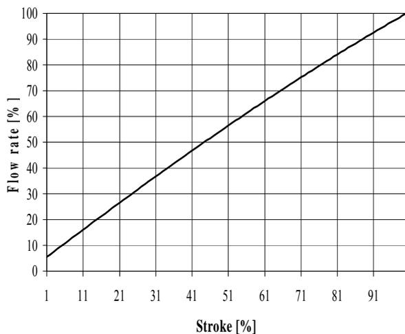
Fig. 7. The work characteristic of the control valve
