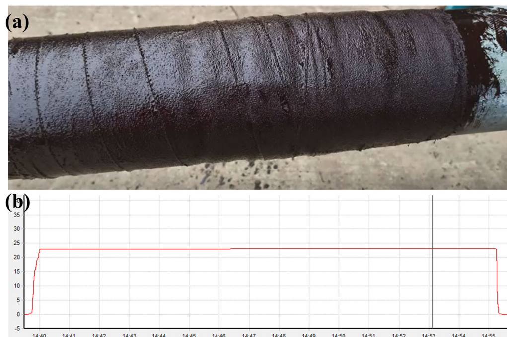
Figure 15. Application experiments on offshore oil and gas well conductors. (a) Curing effect, (b) Pressure retention results.
