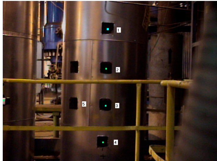
Figure 7. Labeling of measurement points at the level of 17 m.
