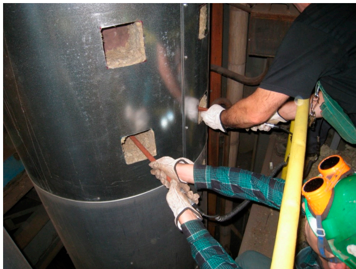
Figure 9. Pipeline vibration measurements at the level of 17 m, unit A.
