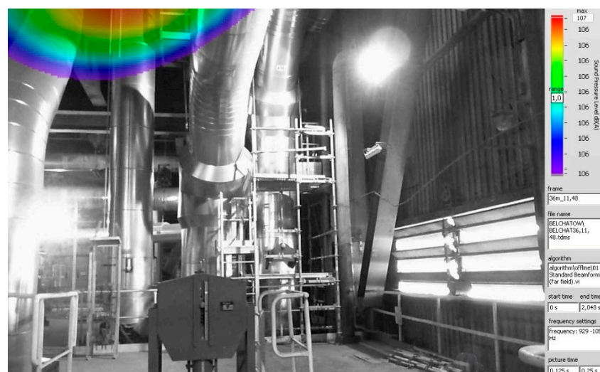
Figure 14. Results of measurements of sound intensity for the frequency range 929 \text{ Hz} \div 1059 \text{ Hz} at the level of 36 m at a distance of 11.48 m from the sound source.
