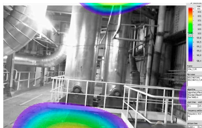
Figure 12. Results of measurements of sound intensity for the frequency range 929 ÷ 1059 Hz at the level of 12 m at a distance of 7.39 m from the sound source.
