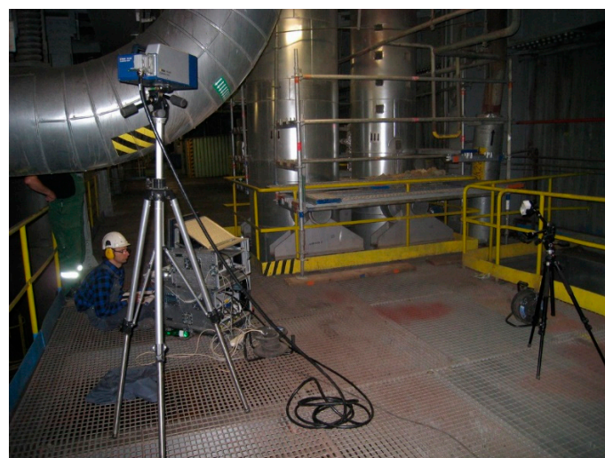
Figure 6. The laser vibrometer system during vibration measurements.
