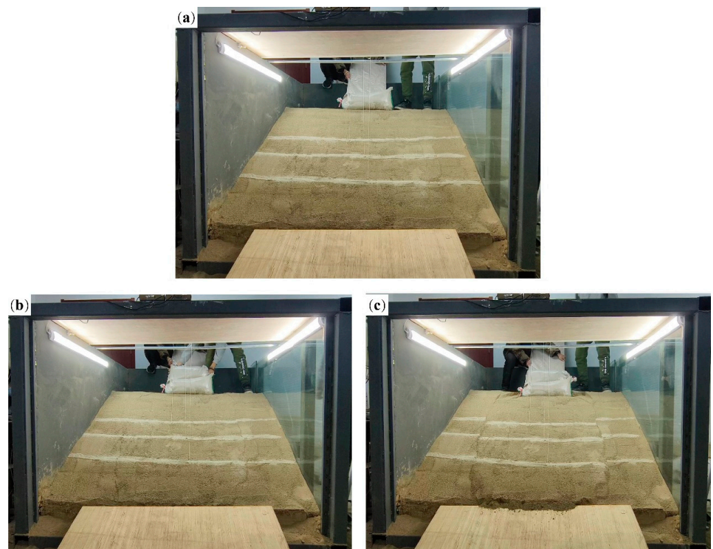
Figure 8. Patterns of crack propagation during the loading process in the Experiment-L: (a) at a surcharge of 30 kg after 1 min and 50 s; (b) at a surcharge of 60 kg after 2 min and 25 s; and (c) at a surcharge of 60 kg after 3 min and 50 s.
