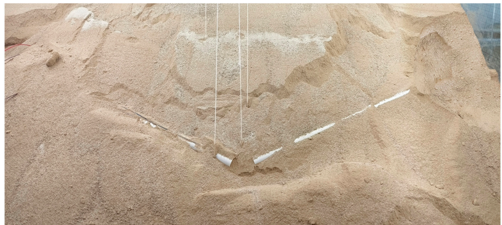
Figure 16. Fracture of the pipeline in the Experiment-LP.
