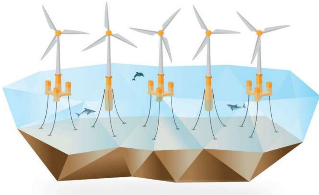
Figure 1: Spar Buoy Platform [1]
