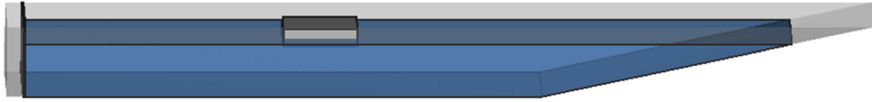
FIGURE 2 | Three-dimensional (3D) model of numerical model. Figure 2 is the 3D model diagram of the numerical model of this experiment. The length of the tank is 4.7 m, the width is 0.4 m, the water depth is 0.3 m, and a wave generator is set on the left side of the tank to simulate the wave environment.
