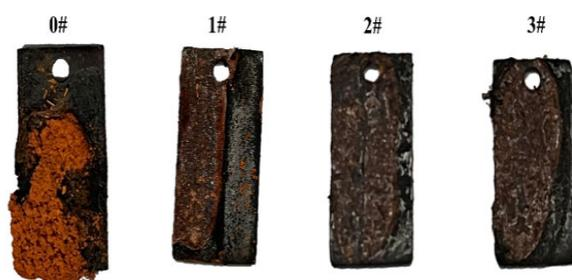
**Figure 1.** Macro morphology of 0#EH36 offshore platform steel, 1#La steel, 2#Ce steel, and 3#Pr steel after 63 d corrosion.
