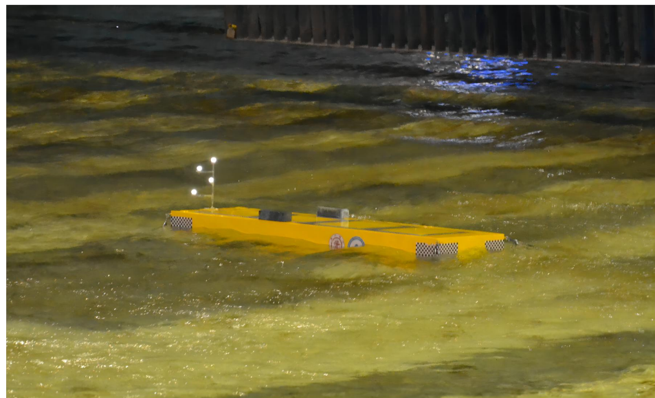
Figure 4. Snapshot of the offshore aquaculture platform within waves.
