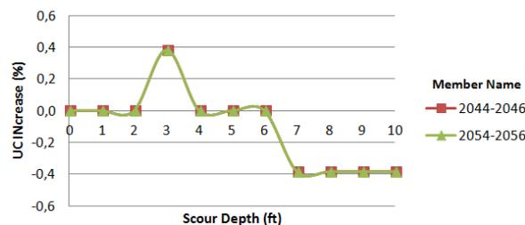
**Figure 16.** Normalized UC Change for Main Deck in Seismic Condition
