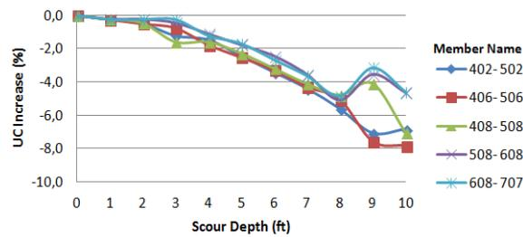
Figure 22. Normalized UC change for pile inside jacket in seismic condition
