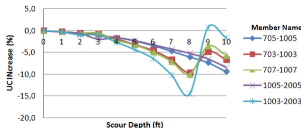
**Figure 18.** Normalized UC change for deck leg in seismic condition
