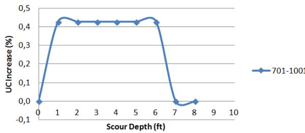
Figure 6. Normalized UC change for deck leg in storm condition
