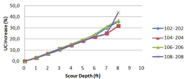
Figure 11. Normalized UC change for pile under jacket in storm condition
