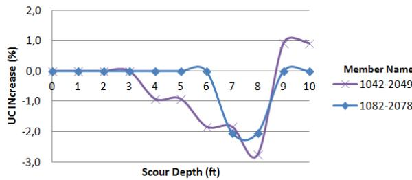
**Figure 19.** Normalized UC change for deck truss in seismic condition
