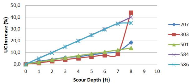
**Figure 13.** Normalized UC change for joint in storm condition
