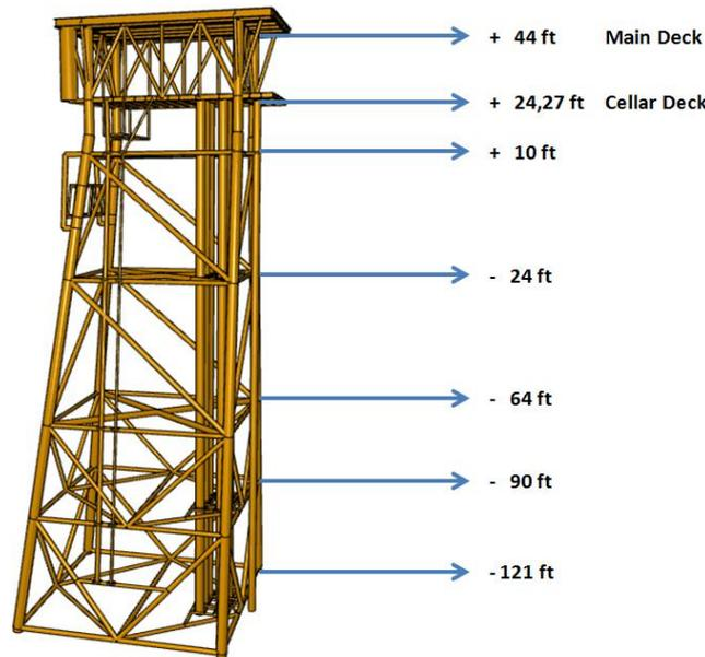
**Figure 1.** Jacket type offshore platform model
