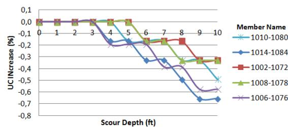
**Figure 17.** Normalized UC change for cellar deck in seismic condition
