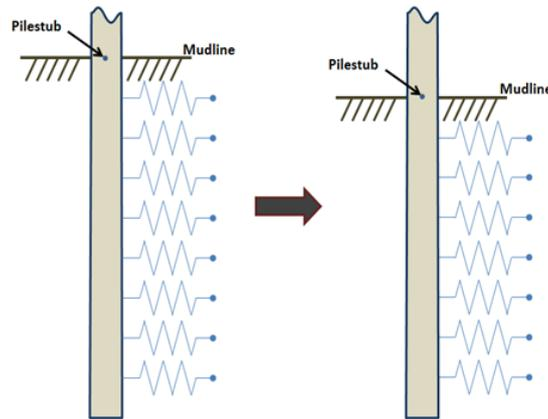
**Figure 3.** Illustration of scour model on the platform's model, showing only pile below the jacket elevation
