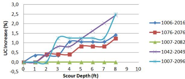
Figure 7. Normalized UC change for deck truss in storm condition
