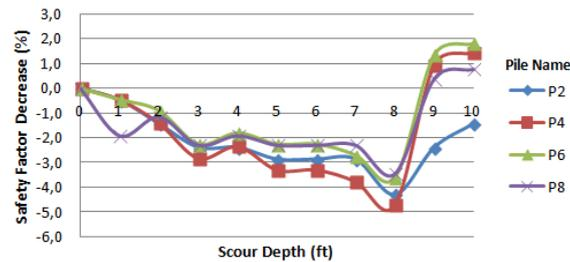
**Figure 25.** Normalized change for pile in tension safety factor in the seismic condition
