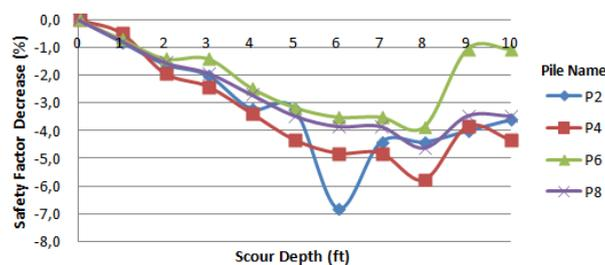
Figure 24. Normalized change for pile in compression safety factor in seismic conditions
