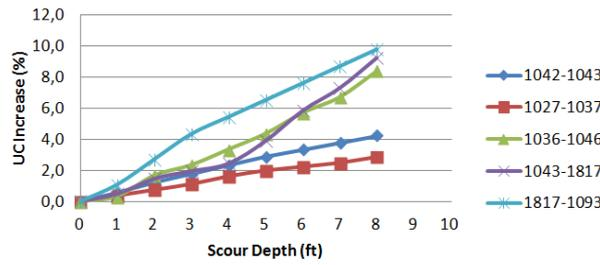
Figure 5. Normalized UC change for cellar deck in storm condition
