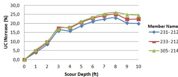
**Figure 20.** Normalized UC change for diagonal bracing in seismic condition
