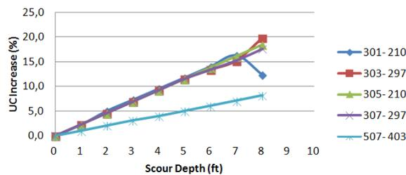
Figure 8. Normalized UC change for diagonal bracing in storm condition
