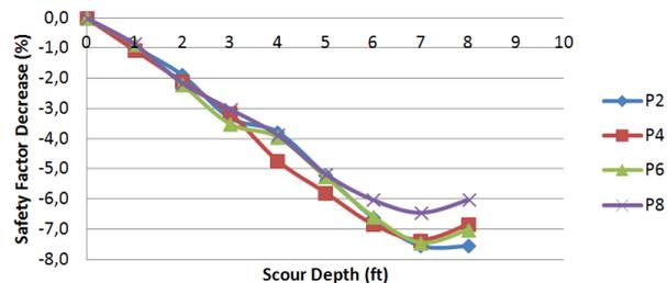
**Figure 15.** Normalized change for pile in tension safety factor in storm condition
