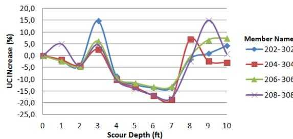
**Figure 21.** Normalized UC change for pile under the jacket in seismic condition
