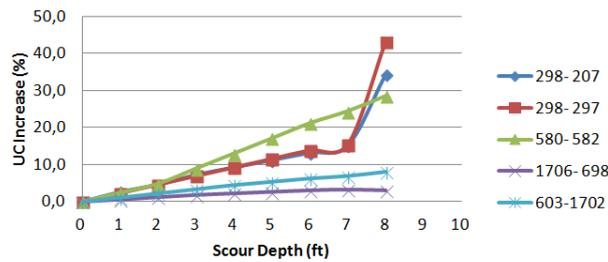
Figure 9. Normalized UC change for horizontal frames in seismic condition
