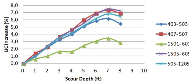
Figure 10. Normalized UC change for leg members in storm condition
