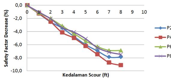
**Figure 14.** Normalized change for pile in compression safety factor in storm condition
