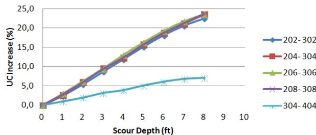
**Figure 12.** Normalized UC change for pile Inside jacket in storm condition
