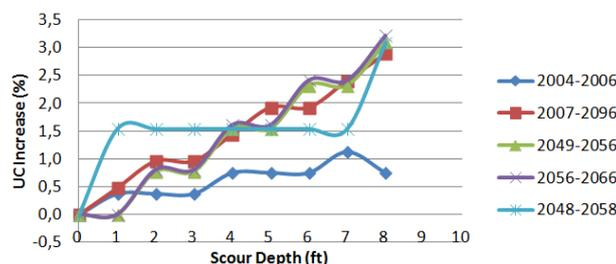
**Figure 4.** Normalized UC change for the main deck in storm condition
