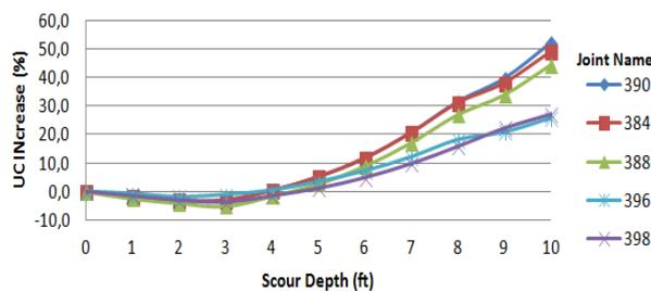
Figure 23. Normalized UC change for joint in seismic condition
