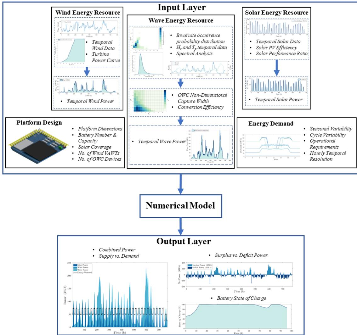
FIGURE 1: A FLOW CHART VISUALISATION OF THE NUMERICAL MODEL PROCESSES, DETAILING THE INPUT AND OUTPUT LAYERS
