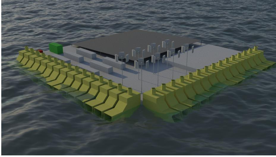
**FIGURE 2: RENDER OF THE CONCEPTUAL PLATFORM DESIGN ILLUSTRATING THE OWC DEVICES, VAWTS, SOLAR PV COVERAGE AND ASSOCIATED INFRASTRUCTURE**
