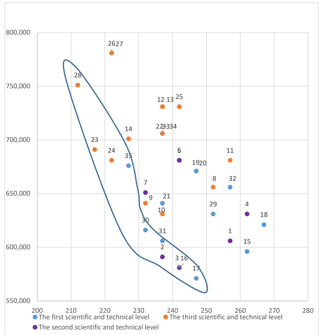
Figure 5. The relationship between life cycle cost and life cycle duration and scientific and technological level of the digital model of the life cycle of an offshore oil and gas platform: on the ordinate axis—the costs of creating a variant of the life cycle of an offshore oil and gas platform, monetary units; on the abscissa axis—the duration of creating a variant of the life cycle of an offshore oil and gas platform, years.
