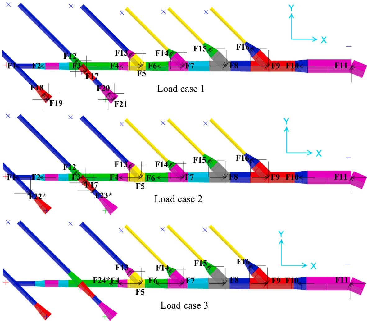
Fig. 9. Forces acting on each member of the model.
