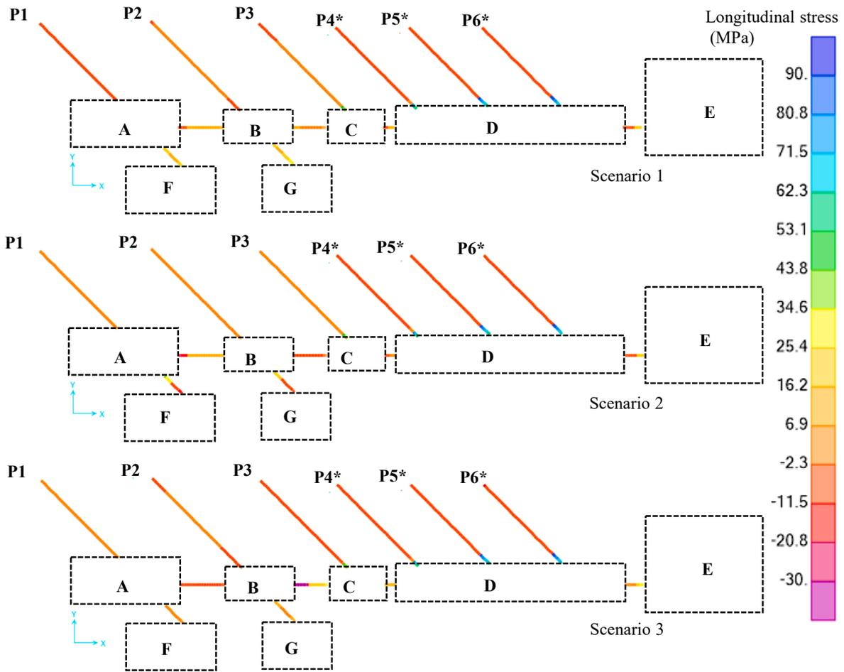
Fig. 15. Transient condition: longitudinal stress for the three scenarios.
