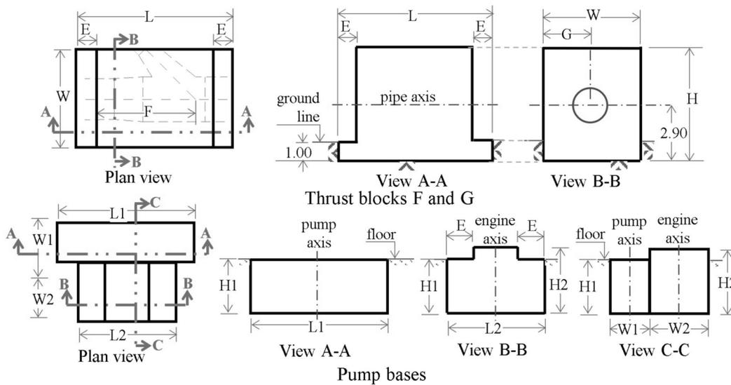
Fig. 6. Geometry description of existing thrust blocks and pump bases.
