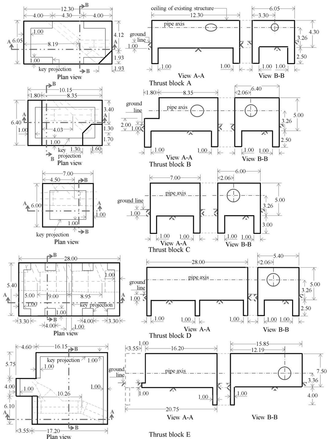
Fig. 7. Geometry description of new thrust blocks, dimensions in meters.
