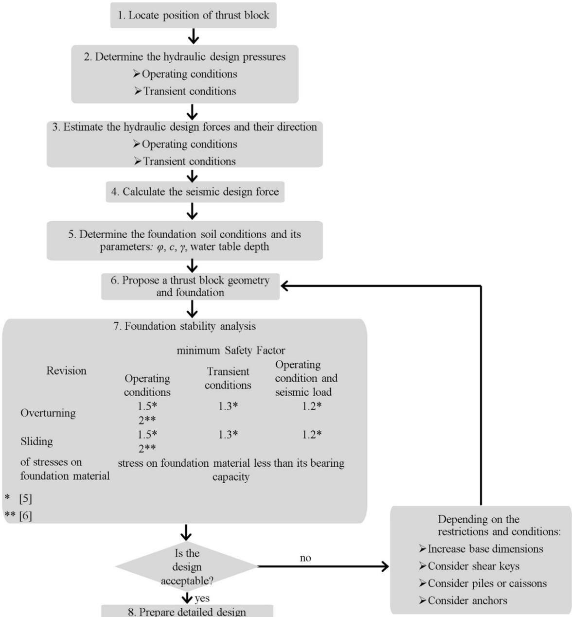
Fig. 4. Steps in the analysis and design of thrust blocks.
