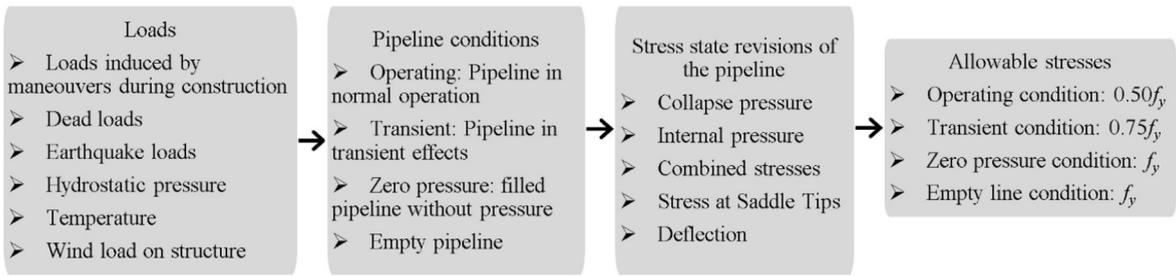
Fig. 3. Steps in the analysis and design of steel supported pipelines according to AWWA [12].
