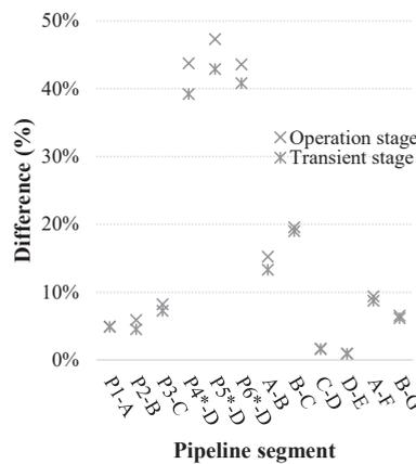
**Fig. 16.** Effect of the structural interaction and the fittings on equivalent stresses.
