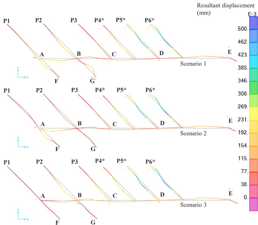
**Fig. 12.** Operating condition: resultant displacement for the three scenarios (scale factor  $\times 5000$ ).
