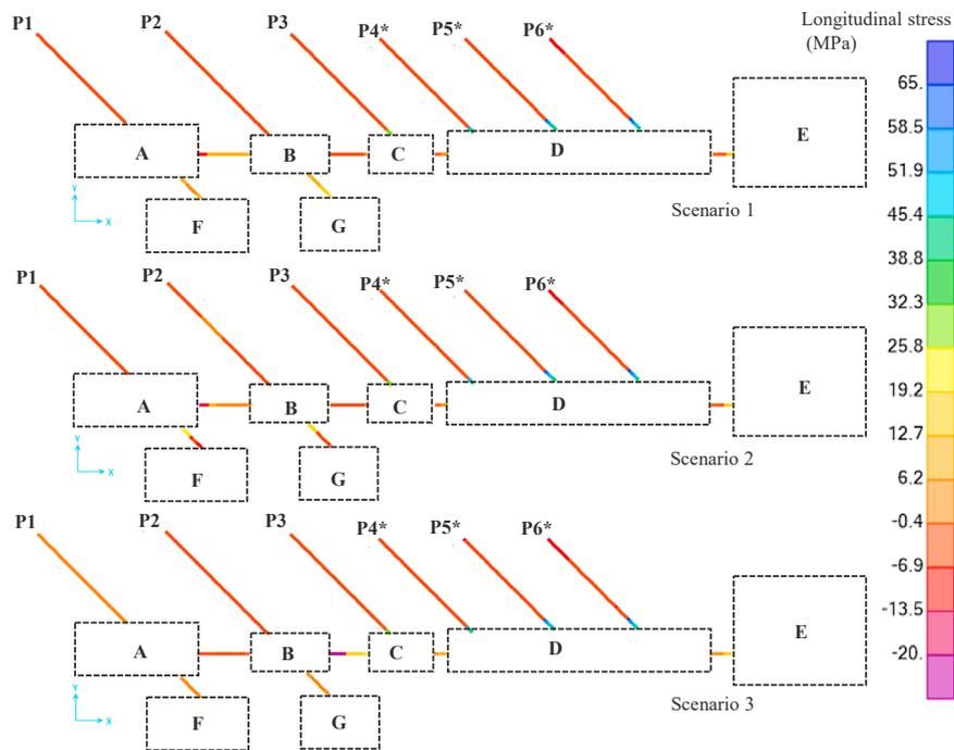
Fig. 14. Operating condition: longitudinal stress for the three scenarios.
