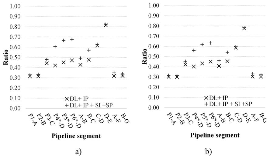
Fig. 17. Comparison between equivalent and allowable stresses: a) operating condition; b) transient condition.
