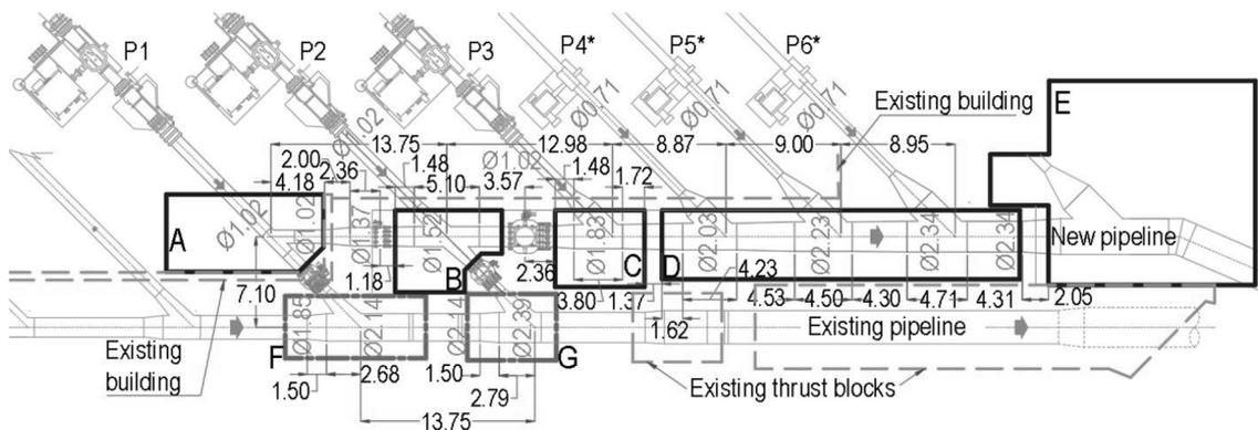
Fig. 2. Model arrangement of the discharge manifolds.
