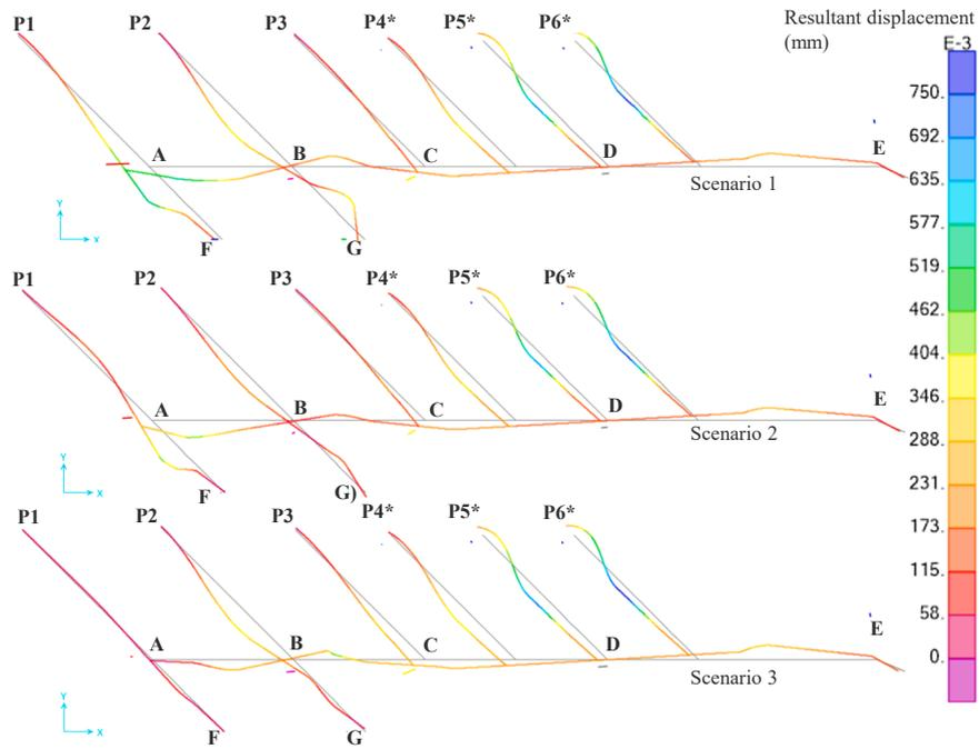
Fig. 13. Transient condition: resultant displacement for the three scenarios (scale factor  $\times 5000$ ).
