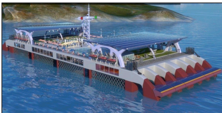
Fig. 30. Semi-submersible wave powered aquaculture cage by Guangzhou Institute of Energy Conversion (Picture courtesy of Mr. Ban Tat Leow).
