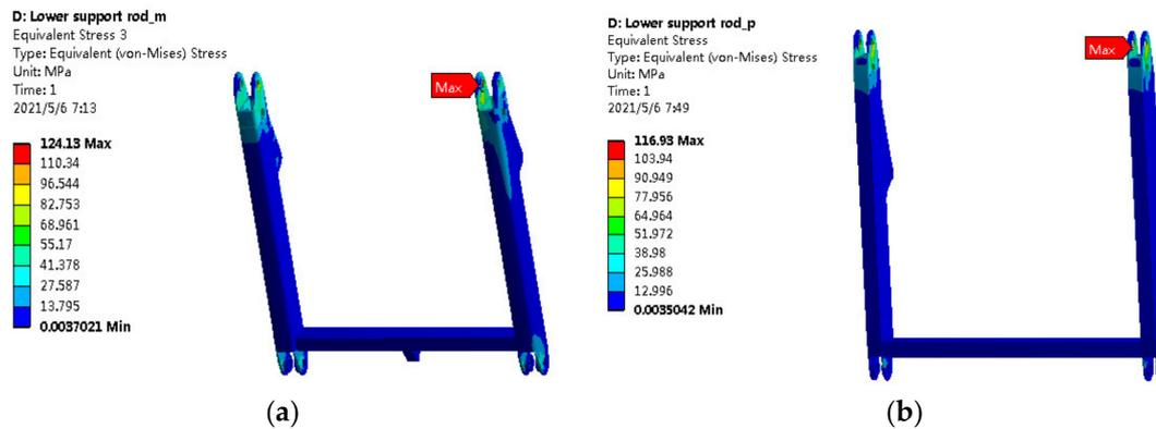
Figure 20. Stress distribution of support components under tensioner support. (a) Scaled model; (b) prototype.
