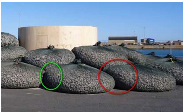
Figure 7 Example of a mock-up test with rock bags overlapping creating a gap underneath.
