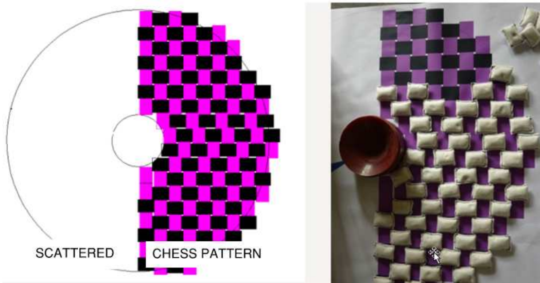
Figure 4 Layout patterns for placement of geobags (right side shows construction in the lab).
