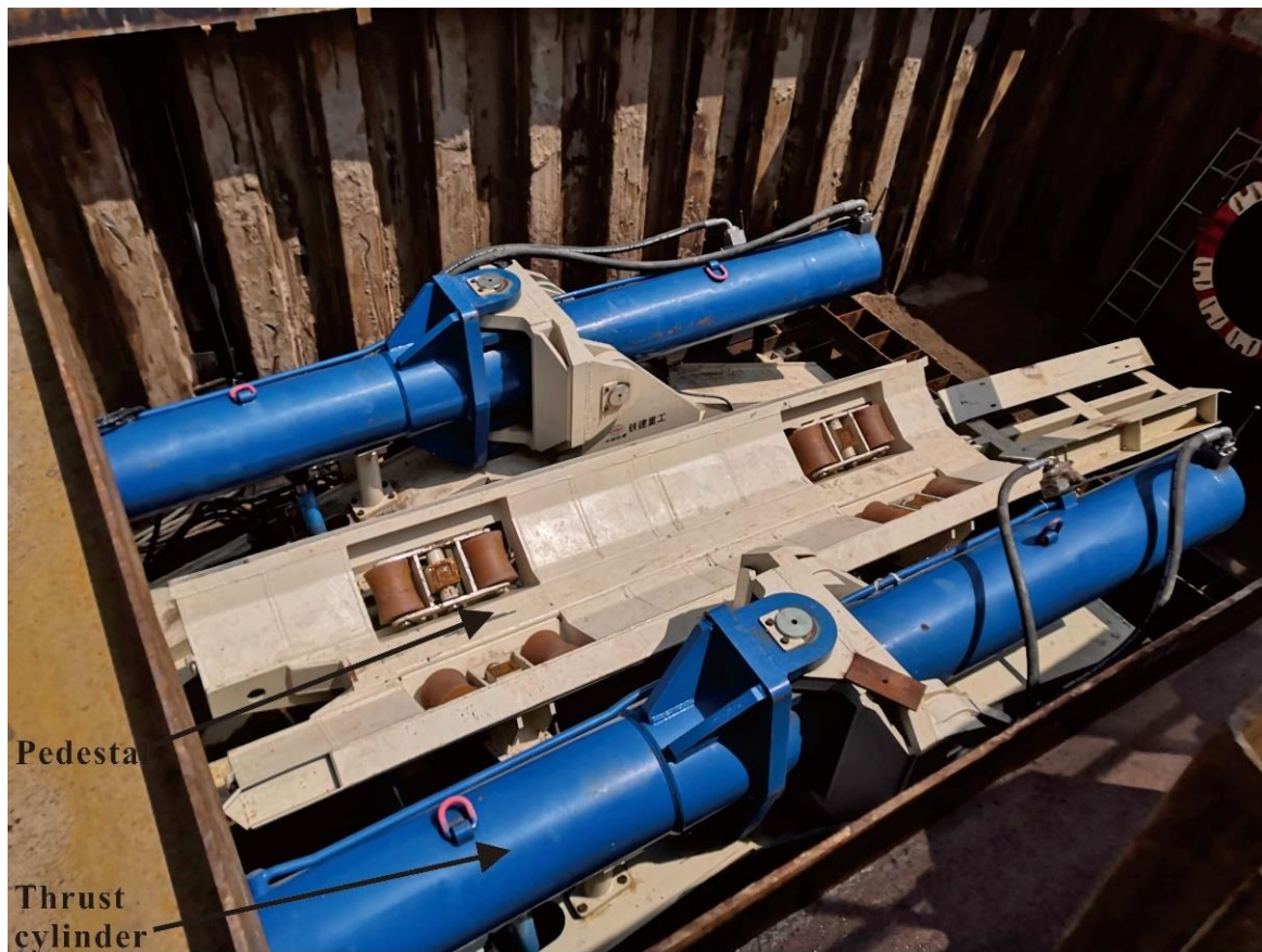
Figure 10. The pedestal of the thrust machine.
