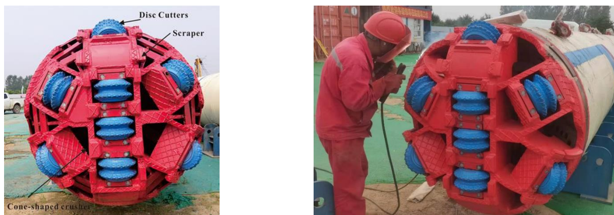
Figure 5. Layout form and modification of cutter head of the boring machine.
