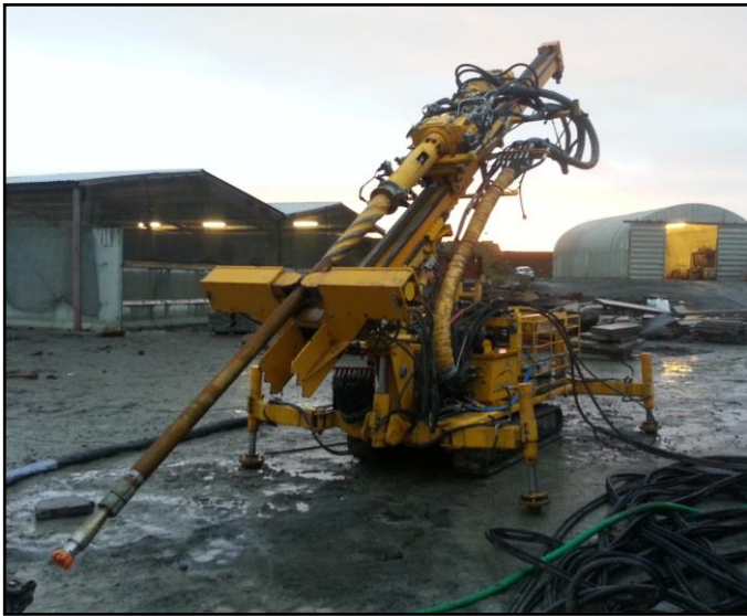
Fig 1: Loaded AROV in rock anchor configuration during land based testing in Orkney
