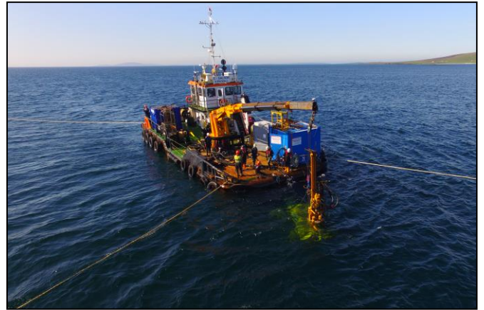
Fig 12: aROV being recovered at slack tide after anchor drilling subsea
