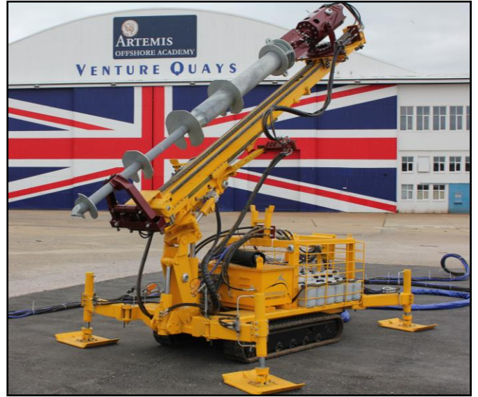
Fig 2: Loaded AROV in screw pile configuration prior to testing at Yarmouth
