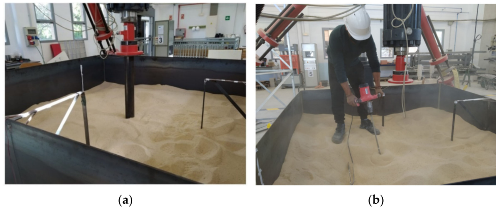
Figure 12. Project phases: (a) testing a pile of 80 mm; (b) decompaction of the sand.
