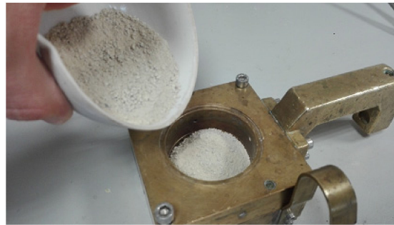
Figure 5. Pouring the sand into the box.
