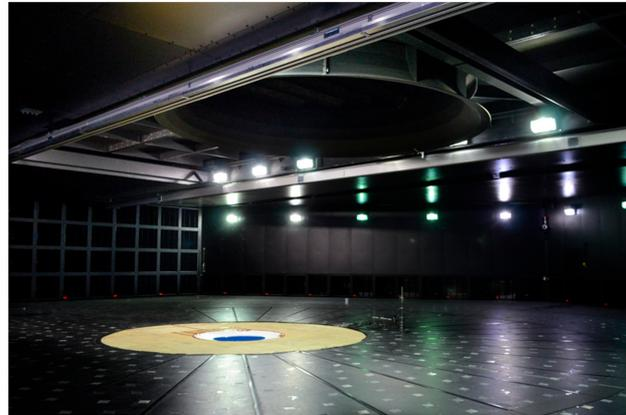
**Figure 1.** WindEEE Dome chamber showing the 60-fan wall and bell mouth (Hangan et al., 2017) [35].
