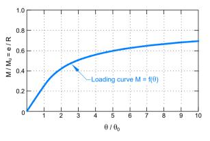
Figure 10.7: Normalised moment-rotation curve – Circular foundation
