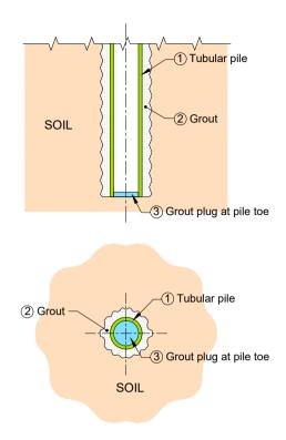
Figure 9.16: Drilled and grouted tubular pile
