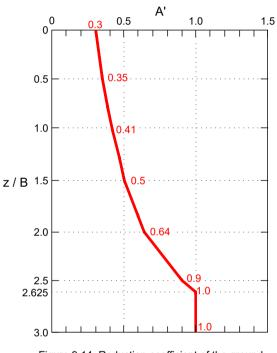
Figure 9.14: Reduction coefficient of the ground reaction P caused by a cyclic loading
