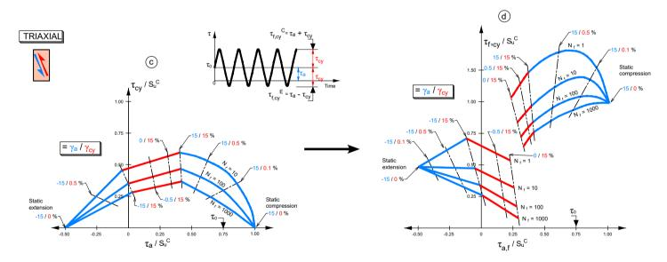
Figure 10.5: Examples of representation of the degradation of shear strength for the whole spectrum of cyclic loading and for different number of cycles, under DSS (a and b) and Triaxial (c and d) loadings, (from Andersen et al., 2013)
