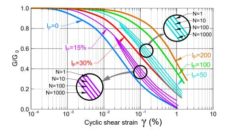
Figure 6.20 : Variation of the normalised shear modulus  $G/G_0$  in function of the level of cyclic strain  $\gamma_{cy}$  for a normally consolidated soil (with a consolidation stress below 150kPa) showing the effect of the plasticity  $I_p$  and of the number of cycles N (from Vucetic et Dobry, 1991)
