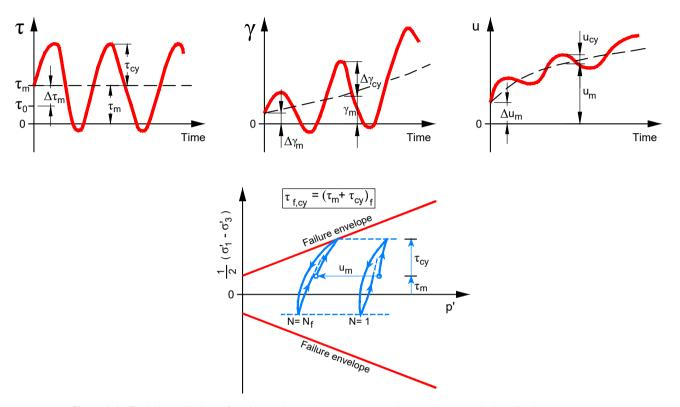
Figure 6.9 : Evolution with time of strains and excess pore pressures in a non-symmetrical cyclic shear test
