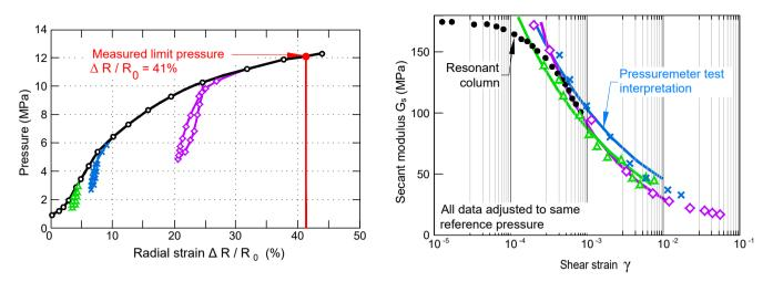
Figure 6.4 : Example of measurement of the shear modulus with a high pressure dilatometer
