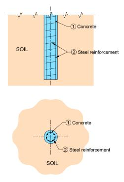
Figure 9.17: Bored cast-in-situ pile with reinforcement
