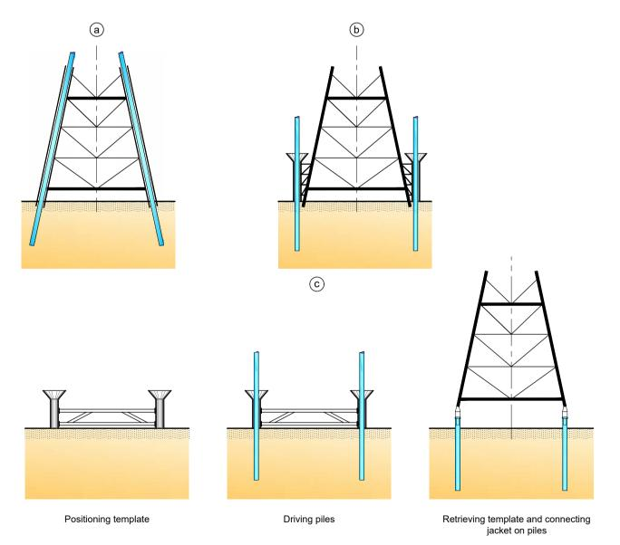
Figure 9.4: Illustration of piles installed in legs (a), in sleeves (b), and through a guide frame (c)
