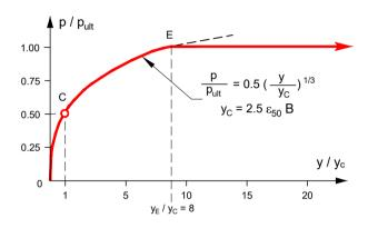
Figure 9.12: Static p-y curves (normally consolidated clays)
