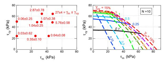
Figure 6.15 : Construction of contour diagrams of distortions (from NGI)
