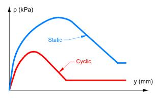
Figure 9.13: Static p-y curves (overconsolidated stiff clays)
