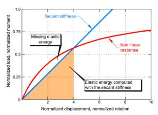
Figure 10.9: Illustration of the underestimation of the elastic energy by taking into account a secant value
