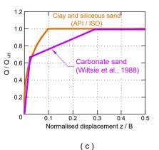
Figure 9.7: Examples of t-z and Q-z curves: (a) t-z curves for siliceous sands and clays (ISO 19901-4, 2016); (b) t-z curves for carbonate sands (from Wiltsie et al., 1988); (c) Q-z curves
