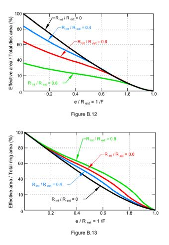
Figure B.13 provides an alternative representation of the previous result, by normalising the effective surface to the total surface of the considered annulus.
