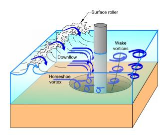
Figure 11.6 : Mechanisms causing scour around a monopile
