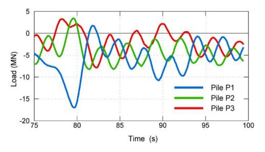
Figure 4.3 : Extreme axial loads transmitted to the head of the three foundation piles of an offshore wind turbine (tripod structure) - Waves with a return period of 50 years
