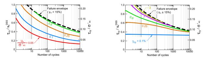
Figure 10.4: Examples of representation of permanent pore pressure (left) and cyclic shear strain (right) in function of the cyclic stress ratio and the number of cycles. Two-way DSS tests (from Andersen et al., 2013)
