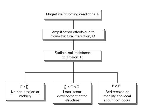
Figure 11.3: Initiation process of scour (from Luger et al., 2017)
