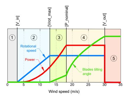
Figure 4.7 : Functioning sketch of a wind turbine in function of wind speed
