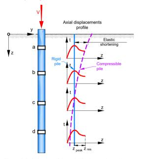
Figure 9.8: Softening of the axial friction and resulting axial flexibility of the pile
