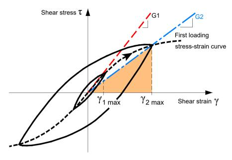
Figure 6.2 : Centred cyclic loading - Direct simple shear test
