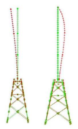
Figure 4.6 : Illustration of 1st and 2nd flexural mode shapes for a wind turbine on tripod
