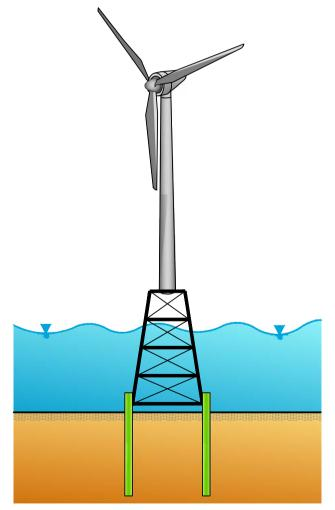
Figure 9.1: Jacket support of a wind turbine - Principle
