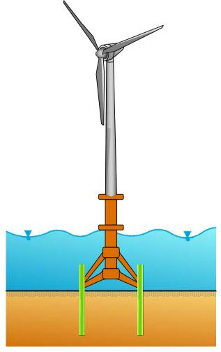
Figure 9.2: Wind turbine support of the tripod type
