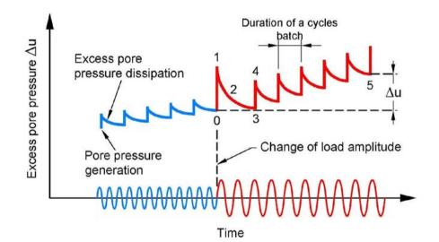
Figure 8.12: Example of generation and dissipation of pore pressure in a soil element (from Taiebat, 1999, guoted by Kirsch, 2014)
