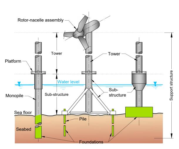
Figure 1.1 : Components of an offshore wind turbine
