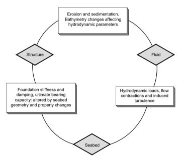
Figure 11.2: Seabed - structure - fluid interaction (from Luger et al., 2017)
