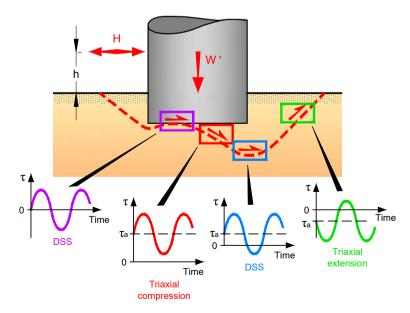
Figure 6.12 : Idealised stress paths for typical soil elements along the potential failure line (from K. Andersen, 2009)
