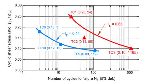
Figure 6.18 : Curves of cyclic shear strength of the N34 Fontainebleau sand for two density indices, with N<sub>f</sub> = number of cycles leading to liquefaction, defined for 5% of axial strain of the sample (from SOLCYP, 2017)
