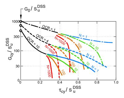
Figure 6.19 : Evolution of the cyclic shear modulus G<sub>cv</sub> (from O'Reilly & Brown, 1991)
