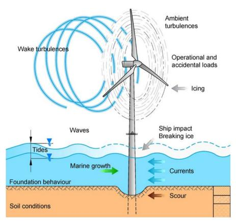
Figure 4.5 : Modelling of an offshore wind turbine
