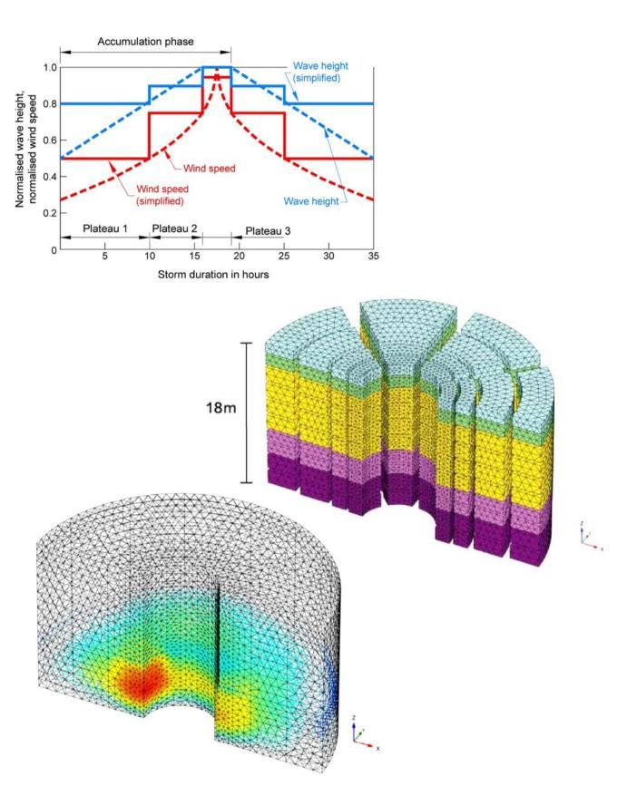
Figure 8.13: Example of accumulation of pore pressures around a monopile (from Kirsch, 2014)
