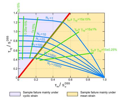
Figure 6.16 Contour diagram of the Drammen clay (OCR=1) obtained from the DSS test (from Andersen, 2009)
