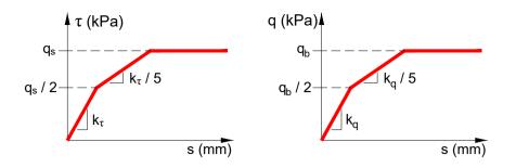
Figure 9.23: Assessment of the axial pile performance based on mobilisation laws of axial friction and end bearing stress according to NF P 94-262 (2012) standard
