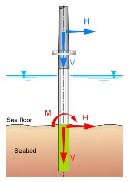
Figure 8.1: Schematic representation of a structure on a monopile
