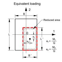
Figure 10.1: Effective cross-sectional area of a rectangular foundation
