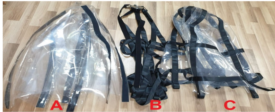
Figure 8. Batychron joining of main components: (A) transparent dome made of TPU material; (B) openwork mesh made of polyester belts; (C) Flexible diving bell—Batychron; Source: Own photos (2022).
