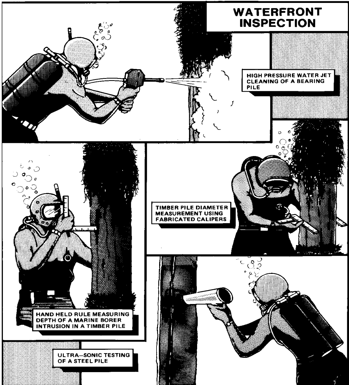
Figure 5-2 Tools and Equipment Used for Waterfront Inspection
