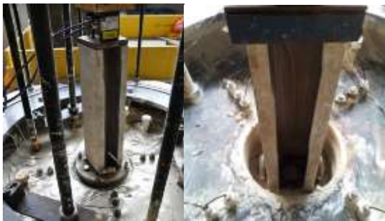
(a) before bearing capacity test (b) after bearing capacity test Fig. 6 Photos of caisson before and after bearing capacity test
