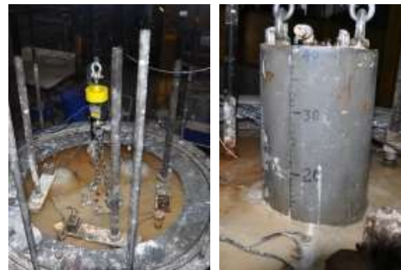
(a) Before pullout test (b) After pullout test Fig. 4 Photos of caisson before and after pullout test
