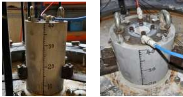
(a) Before installation (b) After installation Fig. 2 Photos of caisson after installation
