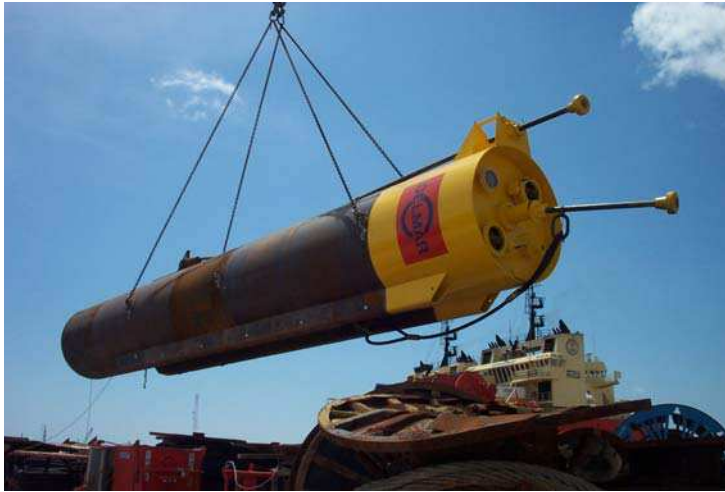
Fig. 10. Suction Anchors for an offshore platform being transported to site in the Gulf of Mexico (Courtesy Prof Aubeny, TAMU).
